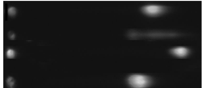
Fig. 2. Raw spectra of four LED's. Spots at left image side corresponds to direct (0 th order) diffraction maxima of LED's and their 1 st order spectra are right (from top: green, white, red and blue LED). Image intensity was numerically increased for better visibility.
