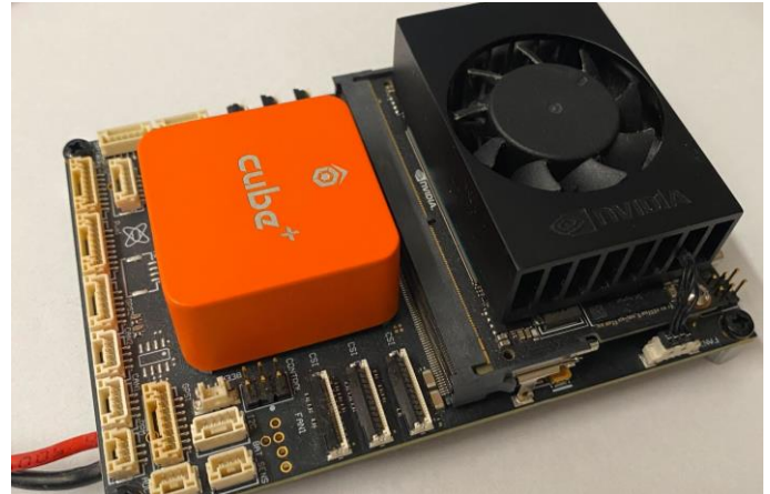
Obr. 4 Airvolute DCS 1.2 s Nvidia Jetson Xavier NX
